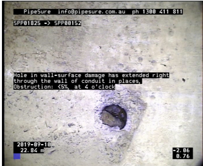
Photo: 1_10A, Media No.: 100919_1, 00:07:49 22.84m, Hole in wall-surface damage has extended right through the wall of conduit in places, Obstruction: <5%, at 4 o'clock
